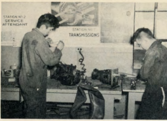
Nez & Marshall Dismantle 3 & 4 Speed Transmission
